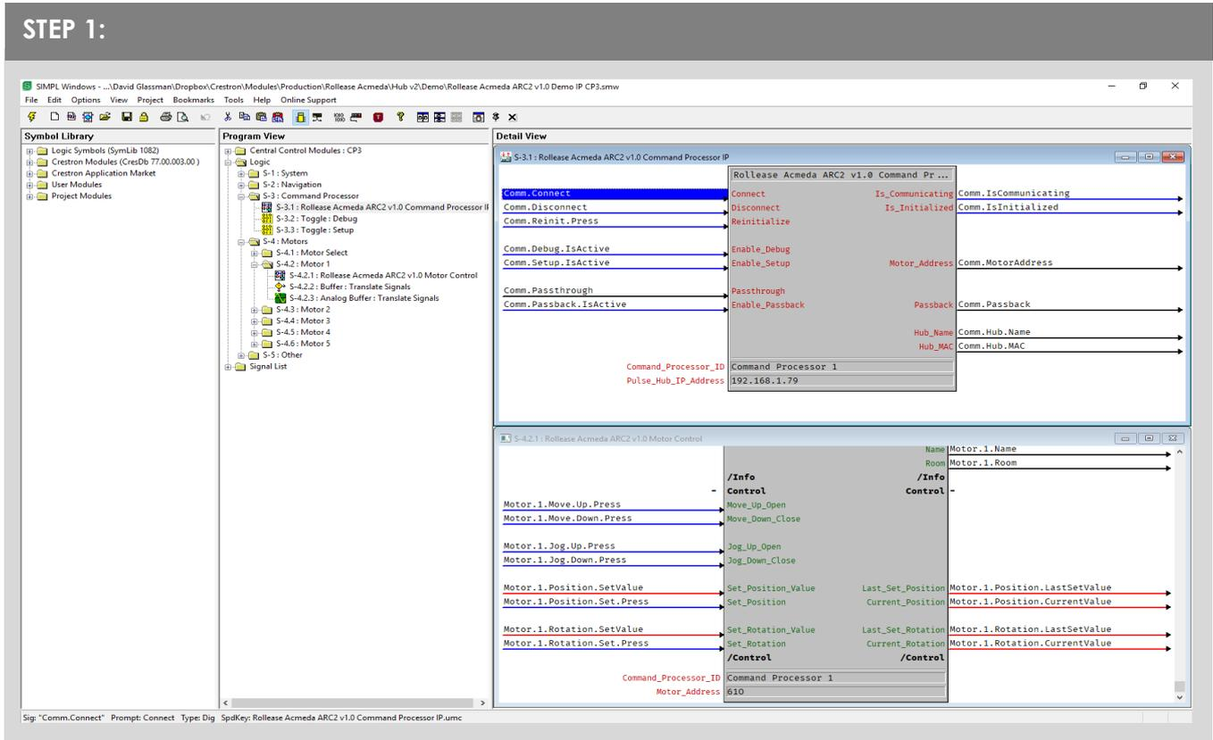
3. Locate the Rollease Acmeda ARC2 v1.0 Command Processor IP symbol in the SIMPL Windows program and replace the current IP address on the Pulse\_Hub\_IP\_Address parameter with the actual IP address of your hub.
