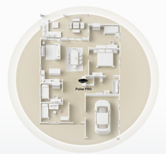
A single Pulse PRO provides seamless control for up to 30 shades in a singlelevel, 3,000 sq. ft. home. For multi-level homes, adding a hub per extra floor ensures reliable connectivity by overcoming signal obstructions.
