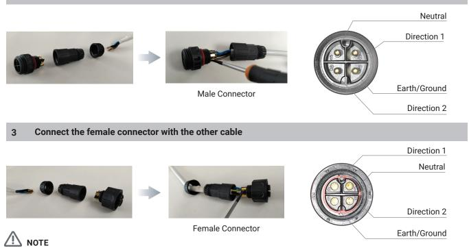
Wires of the same color should be connected to the same number.
