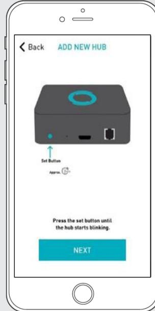
Hold the Wi-Fi Bridge set button for 2 seconds. The bridge will start blinking blue to signify it is ready to pair to the network.
