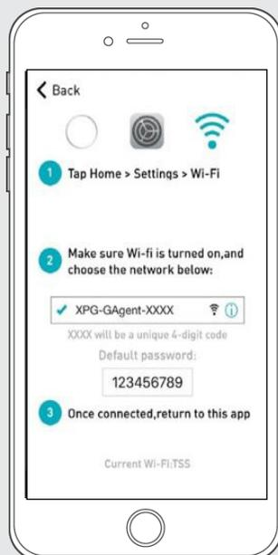
Using your home button exit the Automate Pulse app and enter your Wi-Fi settings. Select the XPG-GAgent-XXXX network and enter the default password 123456789. Return to the Automate Pulse app.
