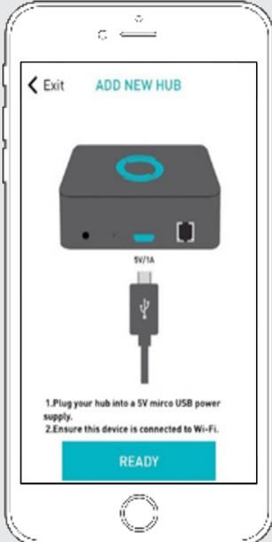
Follow on screen instructions to pair the new Wi-Fi Bridge to the application. Ensure Wi-Fi Bridge is plugged in. Select "Next".
