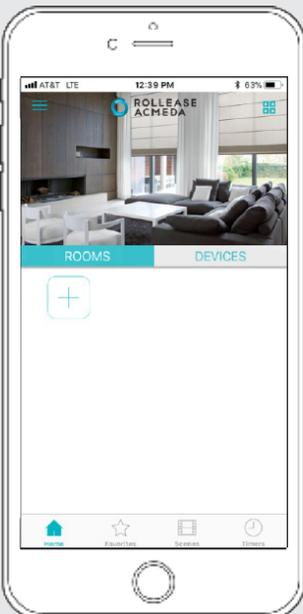
Link the application to the new Wi-Fi Bridge. Select the menu button in the upper left corner of the home screen (3 lines).
