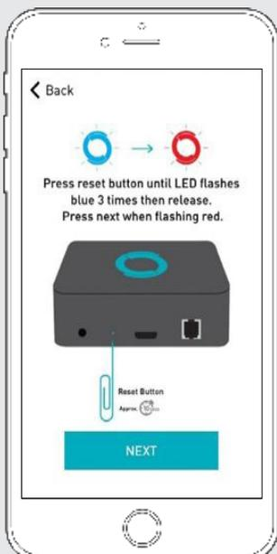
Using a paper clip, press and hold the recessed button on the Wi-Fi Bridge until the Bridge blinks blue 3 times. Press next when the Bridge begins blinking red.
