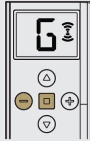
Hold [-] and STOP buttons for 4 seconds. During this time "G" will be displayed. Select a Group from A - E to program. (If no buttons are pressed for 90 seconds the remote will exit out of this mode)
