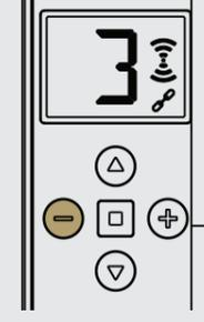
Use [-] button to toggle on/off the inclusion into the Group Channel **Note:** Group Channel Indicator will be shown to indicate Channel is added
