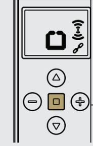
Once desired Individual Channels have been added, press the STOP button to confirm changes. The screen above will be shown for 4 seconds
