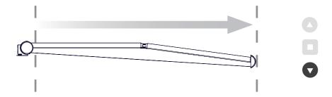
And **UP** on the remote CLOSES the Awning (awning moves in an inward direction).
