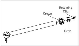
**Step 4.** Slide Motor into tube.
