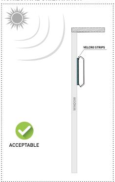
Use velcro strips to stick the bracket on the window (horizontal orientation).
