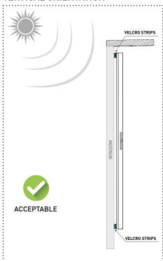
Use velcro strips to stick the bracket on the window (vertical orientation).
