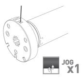
Release **P1** button on motor head.
