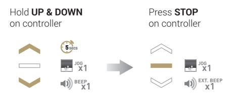
If motor is in Step Mode, use following steps to change to Roller Mode
