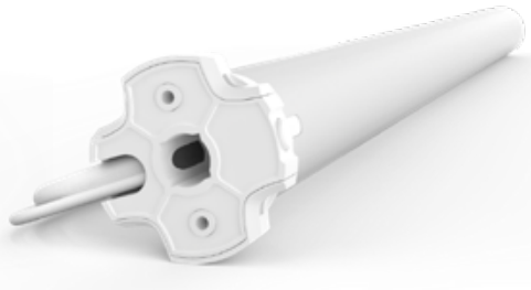
Automate ACRF Q6 110-120 A/C, 6.0Nm, Ø35mm, 24RPM, 21.19in long
