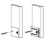
Install CR2430 Battery with positive (+) side facing up.
