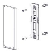
Use supplied fasteners and anchors to attach the hase to wal
