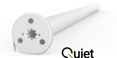
Wire-Free Li-ion Zero Q1.1 5V, 1.1Nm, Ø28mm, 20-28RPM, 649mm long
