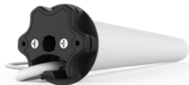
AX50 240V, 50Nm, Ø45mm, 12RPM, 676mm long
