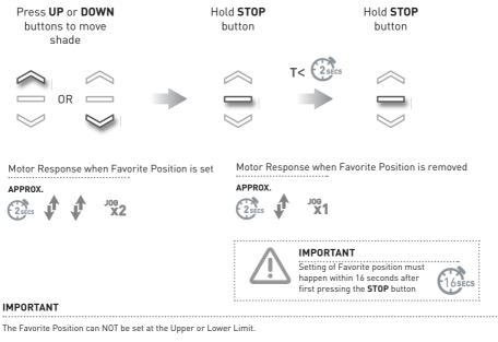
Adjustment of the Upper or Lower Limit will delete the Favorite Position from the Motor and needs to be reset.
