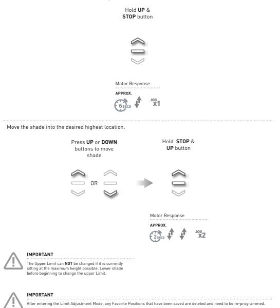
If 4 minutes pass with no button press, the motor will exit the Limit Adjustment Mode and no new positions are set.
