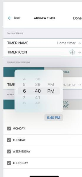
Set the time you wish the timer to trigger shade control to the battery. The motor will jog up and down.
