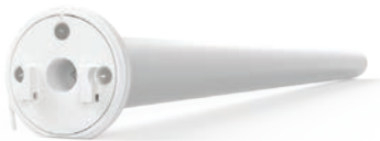
Automate 5V Zero Li-ion Q2.0 5V, 2.0Nm, Ø28mm, 20-28RPM, 25.6 in. long
