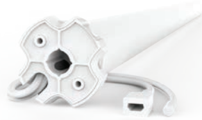
Automate 5V Li-ion 3.0 5V, 3.0Nm, Ø35mm, 20-28PRM, 33.5in long
